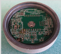
IoT SENSOR PCB IN ITS BOX
